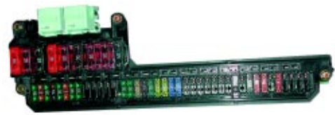
Front Power Distribution Box
